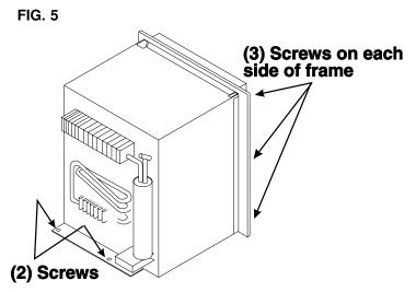
**NOTE**: Push refrigerator into enclosure until front frame is tight against the cabinet. First, secure the frame to cabinet with six screws. Second, install the two screws to the floor at the rear of the refrigerator.
